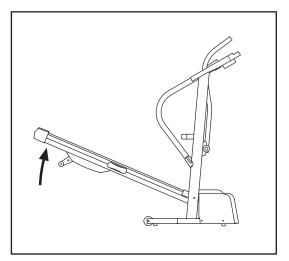
2. Move your right hand to the position shown and hold the treadmill firmly. Using your left thumb, press the storage latch to the left. Raise the treadmill until the storage latch closes over the catch. Make sure that the storage latch is fully engaged over the catch.
